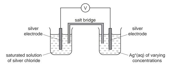
The silver electrodes of the two half-cells were connected via a voltmeter, reading to three decimal places. This measured the cell potential of the concentration cell.
